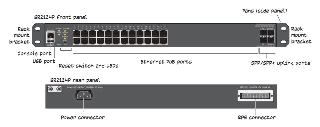
Install the SR2124P switch on a clean, level desktop or surface, or in a standard equipment rack using the rack mount kit that ships with the switch.
